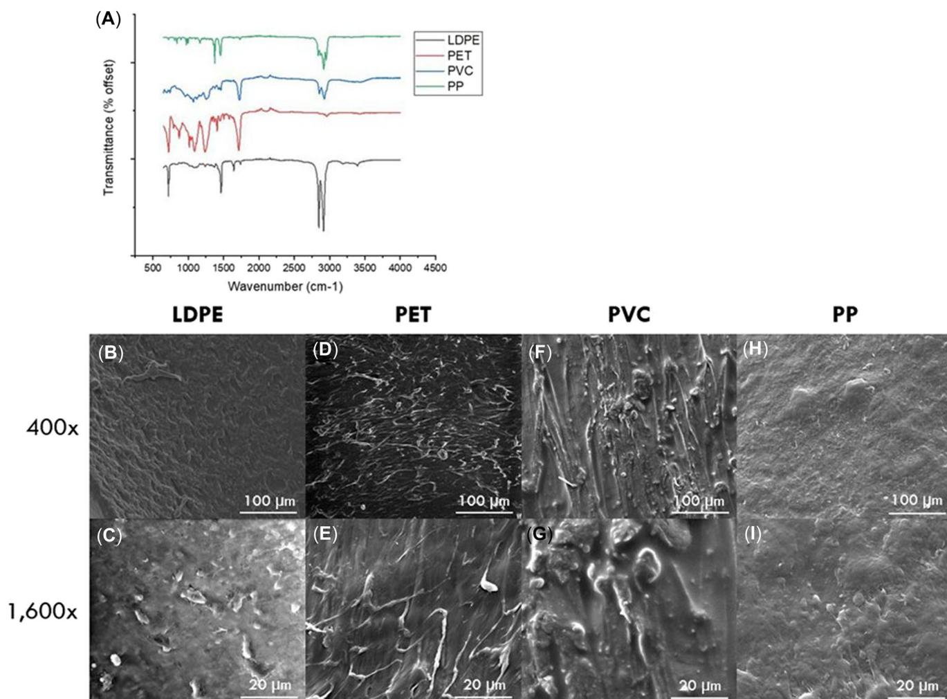
**FIGURE 1:** Fourier transform infrared spectra (A) of low-density polyethylene (LDPE), polyethylene terephthalate (PET), polyvinyl chloride (PVC), and polypropylene (PP). Characteristic peaks were identified and match respective polymer types (Supporting Information, Table S1). Scanning electron microscopy images at  $\times 400$  and  $\times 1600$  magnification of LDPE (B and C), PET (D and E), PVC (F and G), and PP (H and I).
